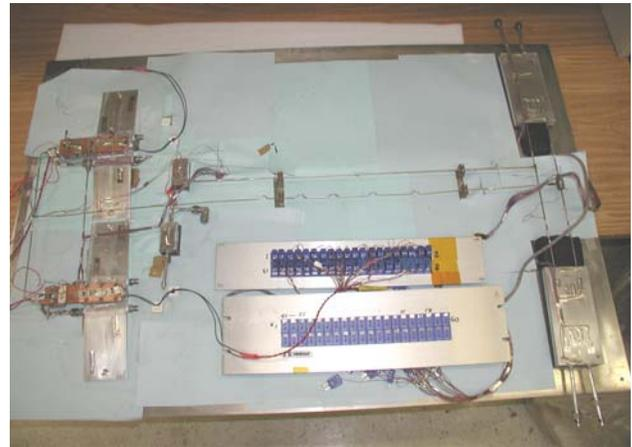
Figure 6. Photo of the MLHP Breadboard.
